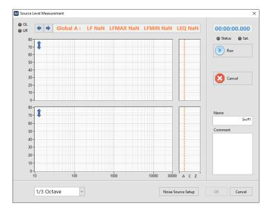
Place the noise source in the source room and turn it ON. When you are ready to perform a measurement, click on the "Run" button or press the top button on the microphone wand.
