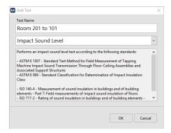
Once the test is created, you can select the standard and enter the receiver room volume:
