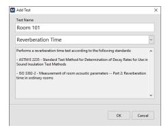
Once the test is created, you can select the standard and select the spectrum type.
