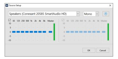
The output setup allows to configure the audio output of the tablet PC to be used as a noise source for the STC tests and RT-60 tests. The generator outputs a pink noise for both audio channels. Two equalizers can be added to customize the sound on each channel. As an example, one channel can be connected to an omni-directional speaker (dodecahedron) while the other can be used with a low-frequency speaker. Hence, two different equalizers can be used for better performance.
