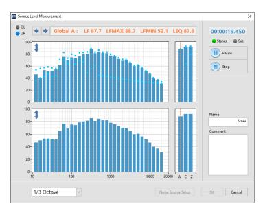
When you are ready to stop the measurement, click on the Stop button or press the middle button on the microphone wand.
