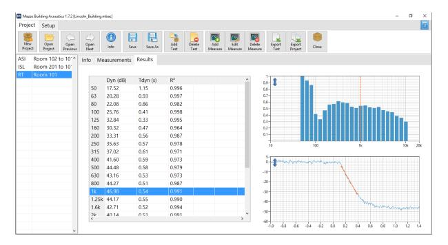
The "Dyn" column indicates the dynamic which is the difference between the source level and the background level. The TX represents the RT-60 reverberation time in seconds and R<sup>2</sup> indicates the correlation coefficient between the measured decay curve and the linear regression curve.
