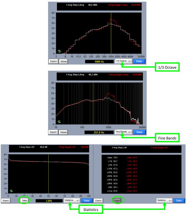
There are two secondary graphs at the bottom of the main interface. Each graph can be set to either 1/3 octave spectrum, fine bands spectrum or statistics (as showed above). The statistics can be displayed either as a graph or as a table with numeric values.
