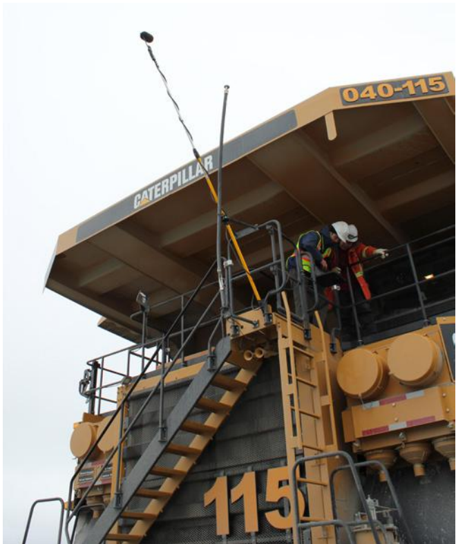
▲ Noise measurements on a moving truck
