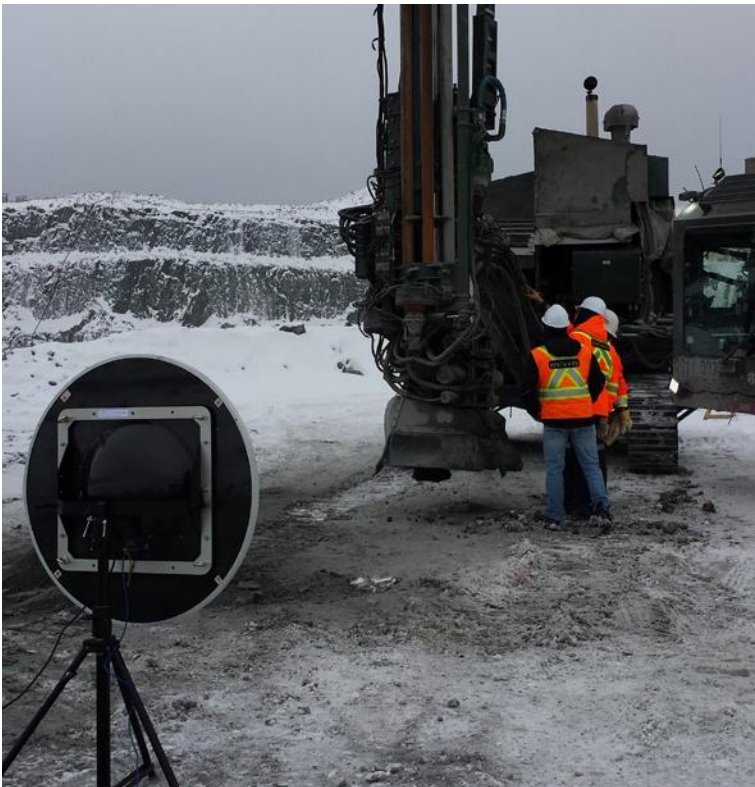
▲ Noise measurements on a drill in winter conditions
