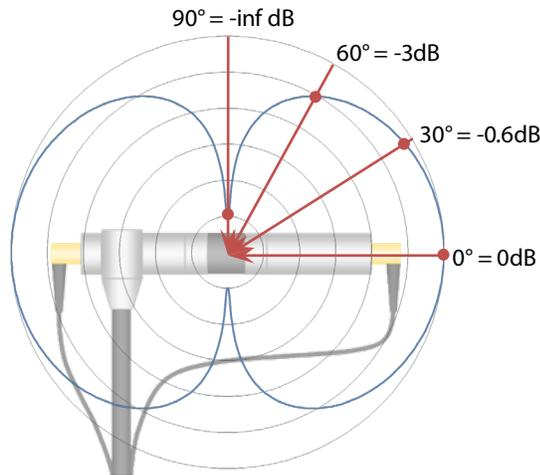
For example, a sound field yielding a sound pressure of 75 dB yields a sound intensity level of 75 dB when the direction of propagation is in-line with the reference axis. It will be 72 dB when the direction of propagation is 60° with respect to the reference axis, and -inf dB when it's 90°.
