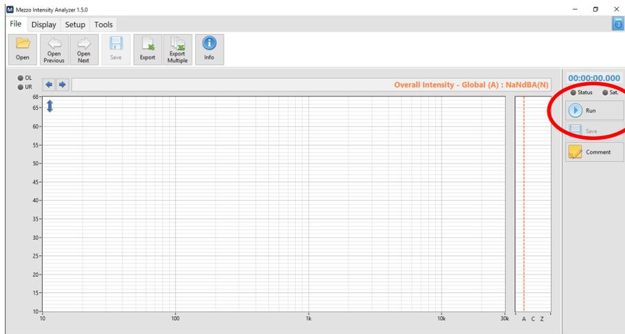
12) As soon as the measurement is started, move the probe at constant speed along the scanning path.
