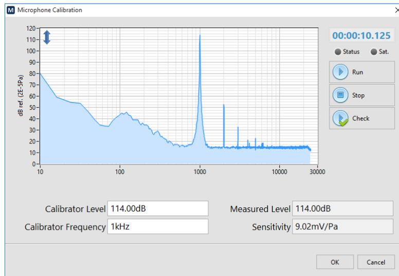
The calibration function will adjust the sensitivity according to the measured level and the calibrator level at the calibrator frequency.
