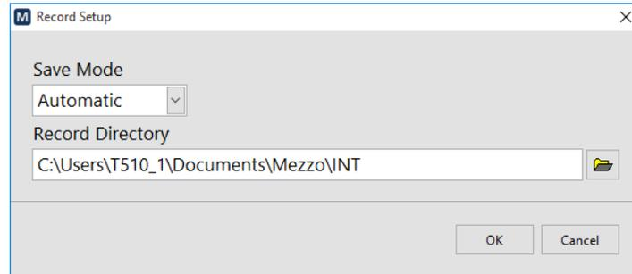
Select the "Automatic" save mode in the drop-down list. The manual mode requires to click the save button once the measurement has ended, whereas the automatic mode records the file automatically at the end of the measurement.
