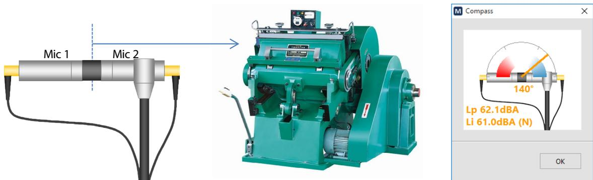
The compass indicator should be in the blue region indicating a PI index inferior to 3 dB and negative intensity.
