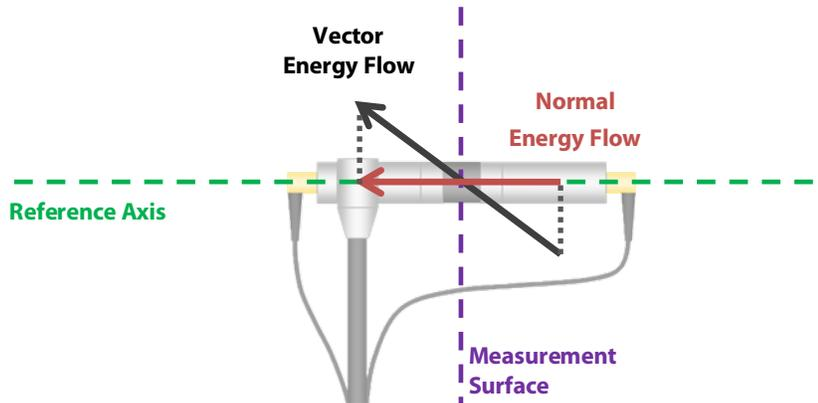
Thus the normal energy flow will equal the full magnitude of the sound intensity vector when the vector is in line with the reference axis. It will be positive when pointing in the reference direction (from mic 1 to mic 2) and it will be negative when pointing in the opposite direction (from mic 2 to mic 1). In addition, a null energy flow will be measured when the vector is perpendicular to the reference axis.
