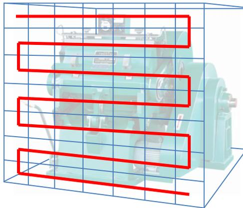
The scanning path must be uniformly distributed on the measurement surface and it must be followed with the probe at a constant speed. For more information on how to select an appropriate path, refer to ISO 9614-2 standard.
