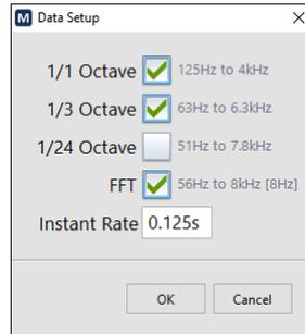
Use the spectrum drop-down list to select from the available spectrum types (1/1, 1/3, 1/24 Octave and FFT). The numbers on the right show the resulting bandwidth. Note that the available bandwidth is affected by the microphone spacer bandwidth. Refer to section 4.1.3, *Selecting the Microphone Spacer*, p. 10 for more information.
