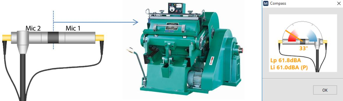
The compass indicator should be in the red region indicating a PI index inferior to 3 dB and positive intensity.
