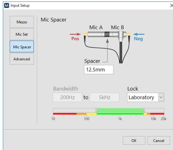
The microphone spacer is an important part of the sound intensity measuring technique using a pair of microphones. Separated by a distance, the two microphones can measure the sound particle velocity by using the pressure gradient. However for this estimation to be right, the separation distance must be adapted to the wavelength. The following table shows the different spacers and their associated bandwidth relative to the degree of precision:
