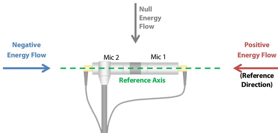
On the other hand, the sound pressure level indicates the sound pressure energy regardless of the direction of the flow of energy. Thus, with the energy flow vector in the reference axis, both sound intensity level will give the same result. However, with the energy flow vector perpendicular to the reference axis, the sound pressure remains unchanged but the sound intensity will be null.
