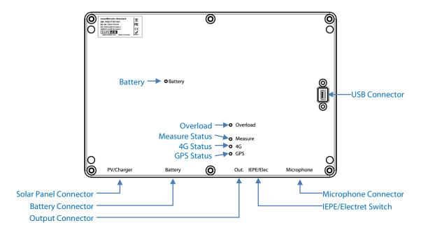
**Solar Panel Connector** – Connect the solar panel cable from the external cabinet connector. The external cabinet connector is used to connect the external solar panel or the power-pack when charging the battery from an outlet or when using the monitoring station indoors.
