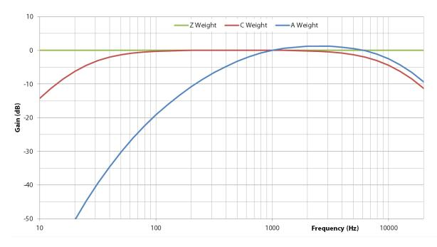
Note that all sound level metrics (SPL, Leq, SEL, Lpk, Lmax, Lmin, and LN%) can be expressed with a specific frequency weighting. For example, the LAeq represents the A-weighted Equivalent Continuous Sound Level.
