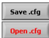
These functions allow saving and recalling a configuration of the data logger. Note that the configuration file does not include the path of the .wav files for both input and output.
