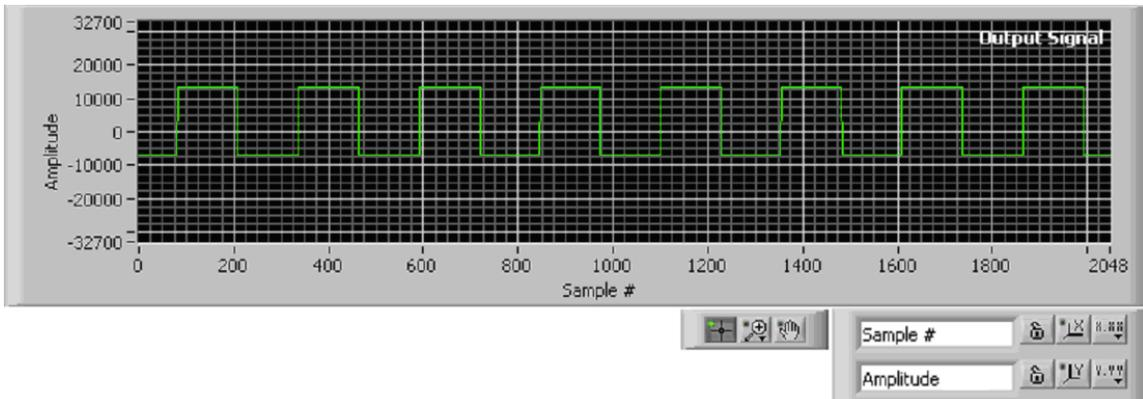
The time signal is in 32-bit format (24-bits right justified: integer values between +8388607 and -8388607). The time signal is presented blocks by blocks (4096 samples). The user can adjust the Y scale by editing the maximum and minimum values directly on the Y scale of the graph:
