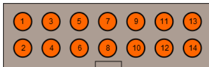
Figure 2 JAi–JBj connector pinouts
