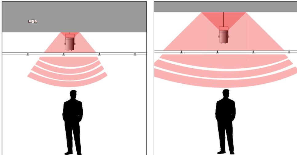
Figure 3: Influence of the plenum height on coverage
