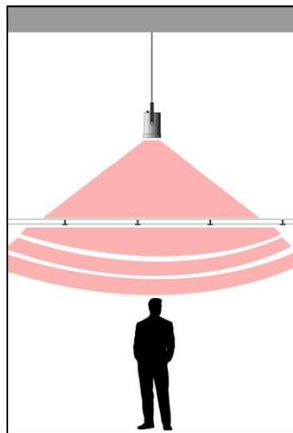
Figure 4: Speakers facing down with very high plenum
