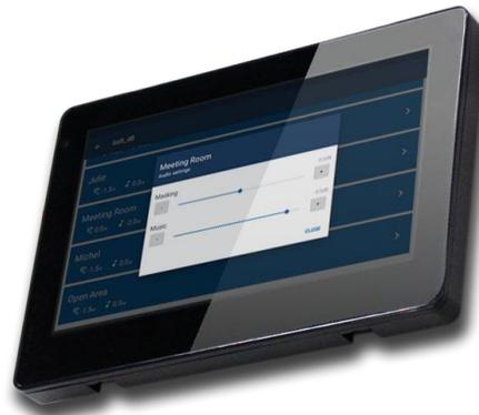
The Control Panel scans the network in search for smartSMS-NET controllers. Upon scanning a Master unit, the Control Panel automatically loads the contained project and displays it in the project list.
