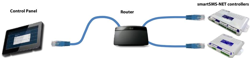
Even though the typical network structure is cabled, a WiFi network would also be appropriate:
