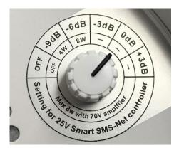
Older models do not have a the "dB" labelling, use the **4W** @ **25V** tap as a default setting with the smartSMS-NET controllers.
