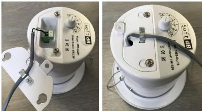
*Note: All wiring should be carried out with 2-conductor stranded copper wire. Typical wire will be 18/2 FT4.*
